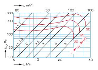
Exhaust valve with angle duct
