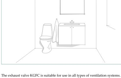
The exhaust valve KGFC is suitable for use in all types of ventilation systems. The valve can be mounted with or without mounting ring. It is ideal for renovation use, because it fits in most round frames and connections. The valve can be ceiling or wall mounted, and the air flow rate is adjustable.
